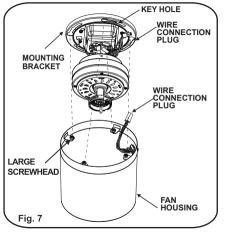
Step 2. Firmly snap the wire connection plug from fan motor assembly to the wire connection plug from fan housing. (Fig.8) Make Sure the wire connections are not in the way of the housing as you lift the housing and proceed to next step.
